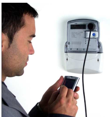
Fig. 28: Meter readout via an IR optical interface
