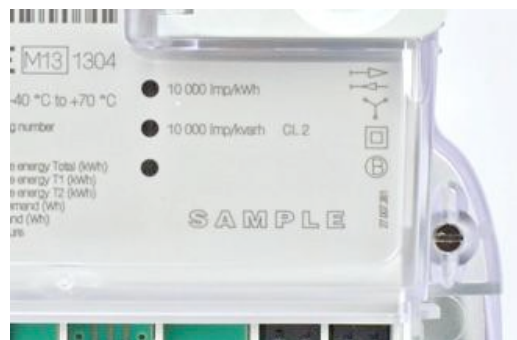
Figure 48: LEDs at MT381 meter
