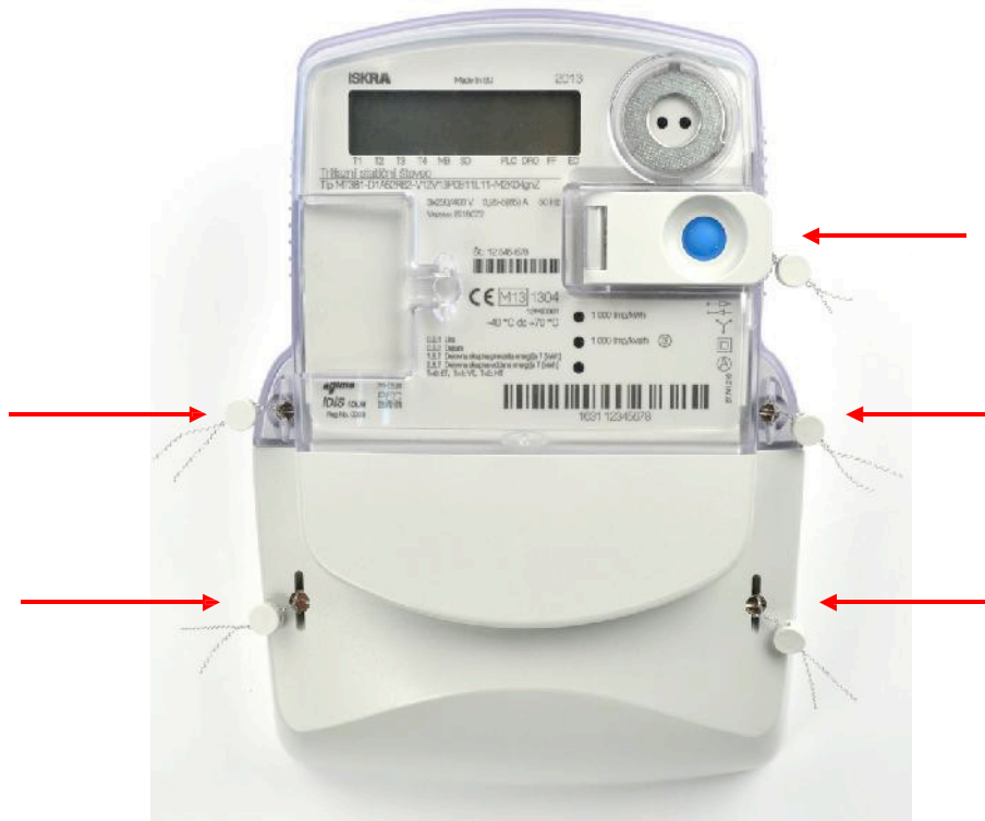
Figure 30: Positions of the seals at MT381 meter
