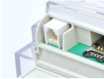
Figure 70: P1 port connection
